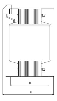
Technical data : Input 400.V at 50/60 Hz and Output 230.V
